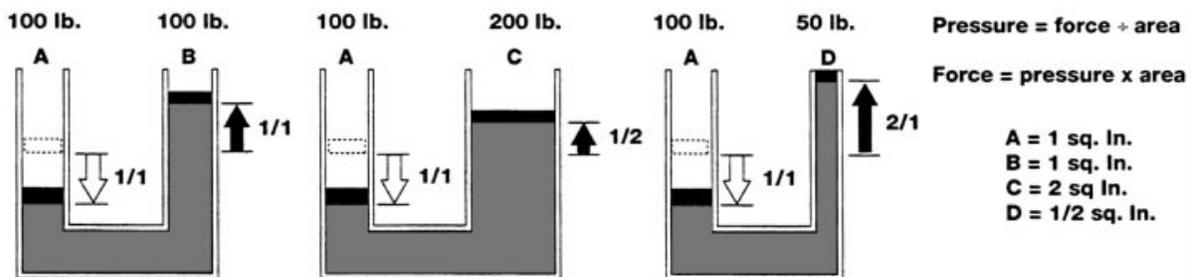
Hydraulic brakes deliver equal braking force to all wheels with a minimum of transmission loss. Hydraulic brakes have a wide design flexibility because braking force can be changed merely by changing the diameter of the master cylinder and wheel cylinders.
