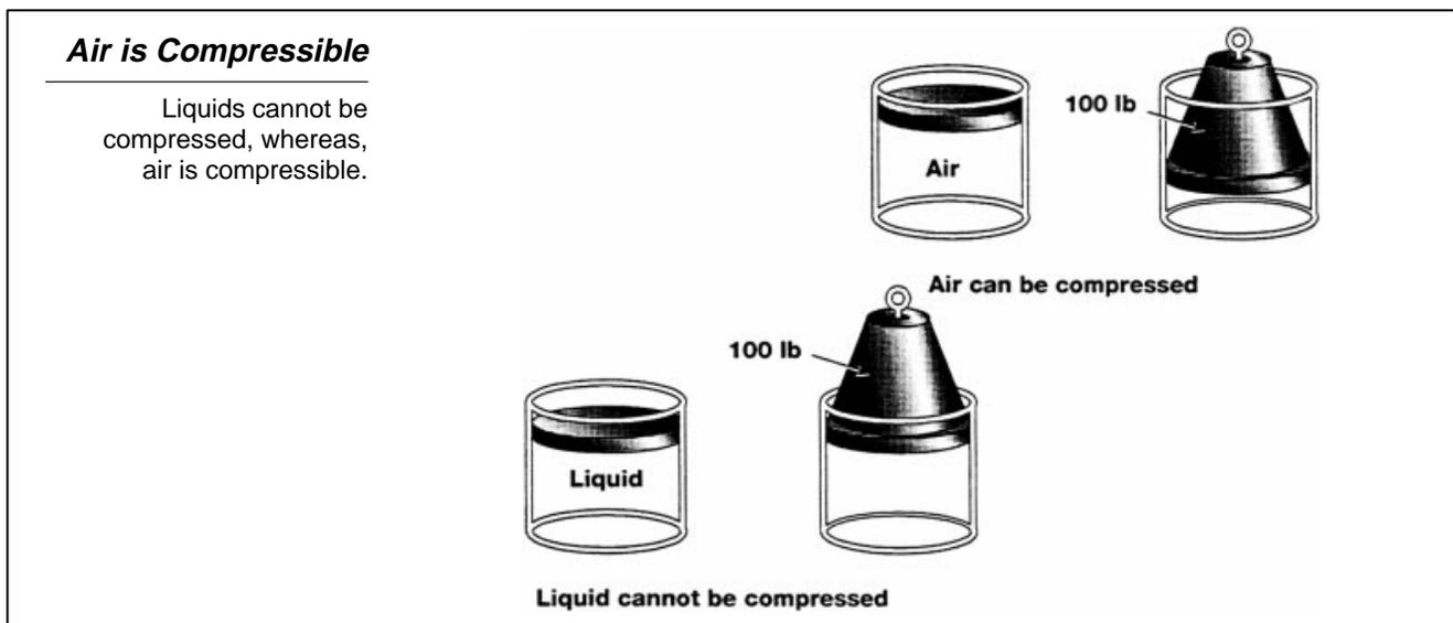
Fluid pressure is indicated in pounds per square inch (psi). It is determined by dividing the input force applied to a piston by the area of the piston. (force/area = pressure in psi) If a force of 100 pounds is applied to a master cylinder piston, an area of 2 square inches, the resulting pressure will be 50 psi. This pressure is transmitted to all parts of the fluid in the container equally.
