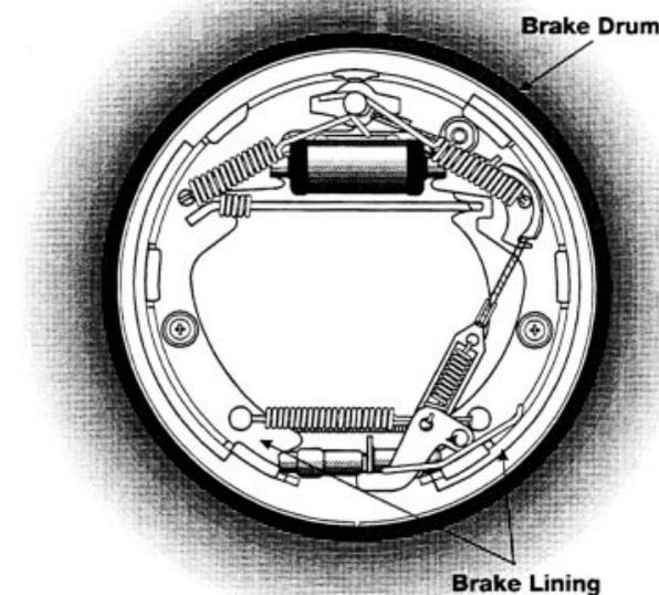
Lining fade affects both drum and disc brakes and occurs when the friction material overheats to the point where the coefficient of friction drops off. When the coefficient of friction drops off, friction is reduced and the brake assemblies ability to convert added heat is reduced.
