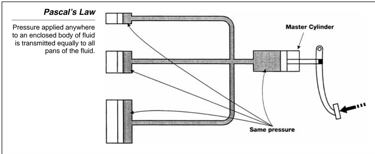
Another important distinction to make is that liquids cannot be compressed, whereas, air is compressible. A hydraulic system must be free of air in order to function properly. Pedal travel will increase as air in the system is compressed.
